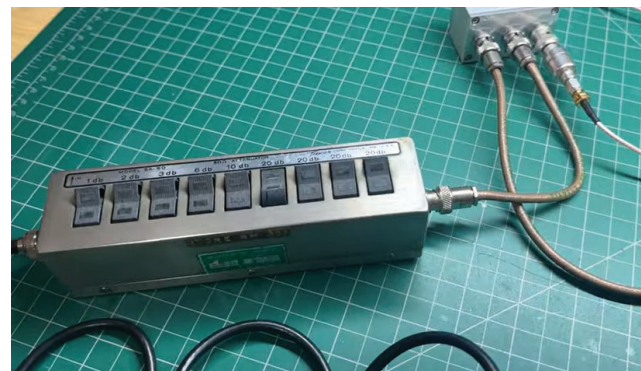
Figure 6 — A 20 dB attenuator helps ensure the signal isn't overloaded.
